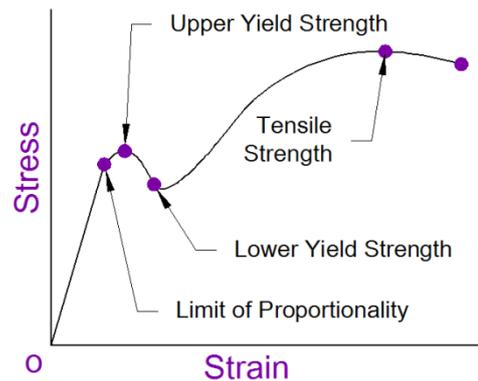
Figure 1.6 - Stress Strain Graph
