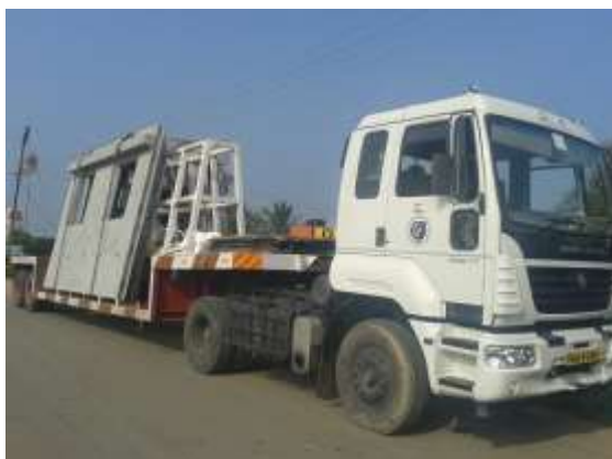
Transporting Wall Panels
