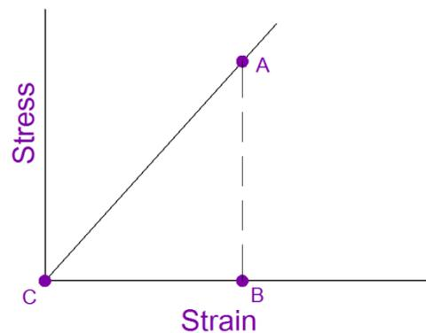
Figure 1.9 – Modulus of Elasticity = AB/BC
